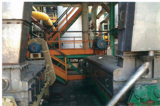
Figure 8: Babbini's fine pulp presses ( P30BC + P40BC)
