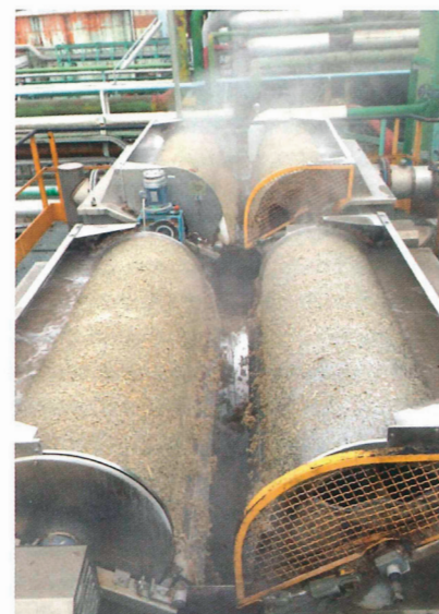
Figure 9: Fine pulp separators from press water
