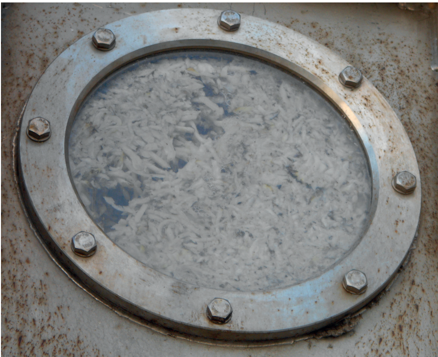
Fig. 5: Empty spaces without spent pulp in the feeding hopper
