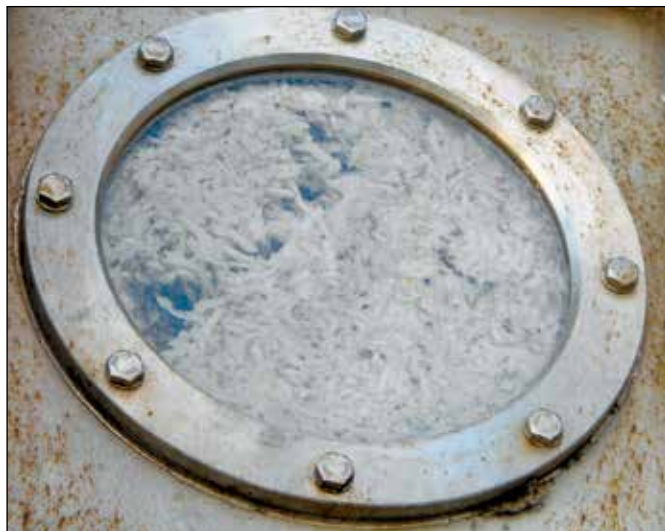
Figure 5. Empty spaces without spent pulp in the feeding hopper
