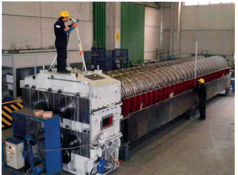
Fig. 3: Pre-assembly of the presses in the workshop
