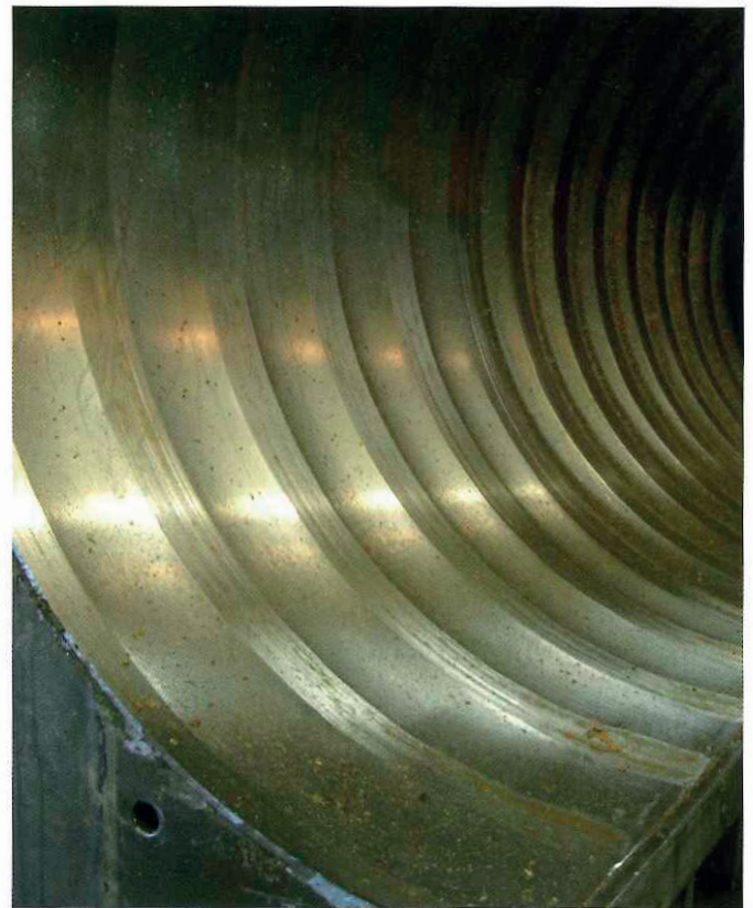
Fig. 10: Cage screen plates deformed by holes clogging
