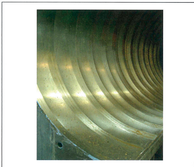
Figure 10. Cage screen plates deformed by holes clogging
